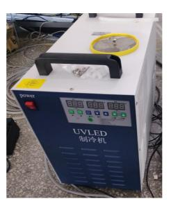
Connect the cooling circulation tube to the water hose. Then open the water-IN valve. Connect the power unit to 220V power and start the chiller working. Finally add the pure water(temp above  $10^{\circ}$ C) or anti-freezing water (temp under  $10^{\circ}$ C)
