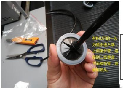
The side marked with inlet connects to the sub-tank, and the other side connects to the printhead.
