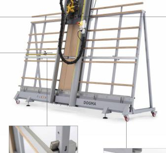
Reference bar mounted on a practical millimeter scale for fast and precise cuttings
