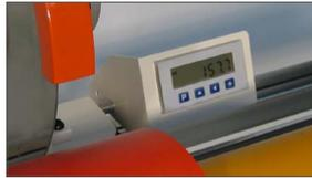
Digital display for cutting measurement
