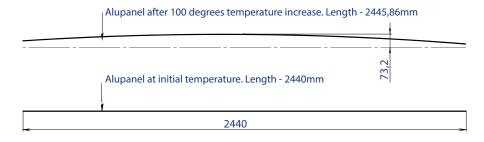
Sometimes it may happen that a substrate on which Alupanel is designed to be installed is rigidly fi xed without taking thermal expansion into consideration. In this case this substrate can bow and deform causing subsequent bowing of the Alupanel fi xed to this substrate. To prevent this substrates on which Alupanel is going to be installed shall be carefully examined.
