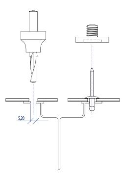
Problems with thermal movements often happen when a panel is fixed to the subframe with rivets or screws. To prevent this, special tools shall be used during such installation.
